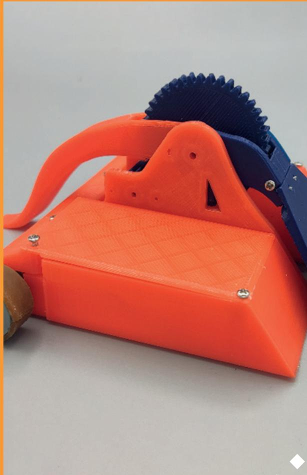
*Two fully 3D printed mini-robots, built from the robot design and complete with the electronics and programming needed to control them.*
