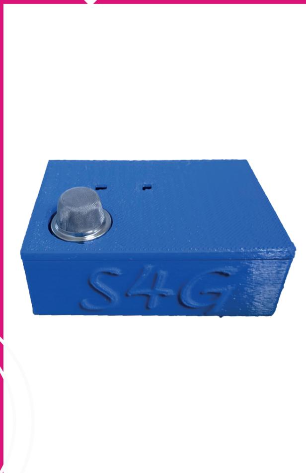
***Zefiro** is a device that carries out air quality measurements. The data is sent to a server that saves it in a database and can be viewed via a web interface.*
